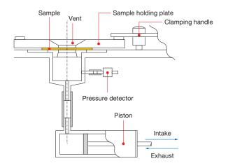
The KES-F8 sends air at a constant flow rate to the sample through the movement of its plunger and cylinder piston. Air can be either discharged through the sample to the atmosphere or sucked in from outside. The pressure when discharging or suctioning air is detected, and the ventilation resistance of the sample (R) is calculated.
