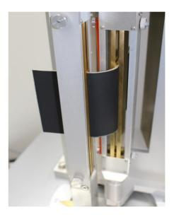
Accurately and quickly measures factors related to curvatures in small bending moments (bending hardness and recoverability).
