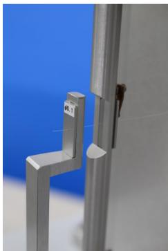
Bending rigidity and recoverability of single yarn and hair can be measured.
